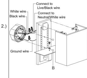
Step2:Wire fixture to wires in outlet box. Copper wire is for Ground.Attach canopy to mounting bracket and tighten with ball nuts.
